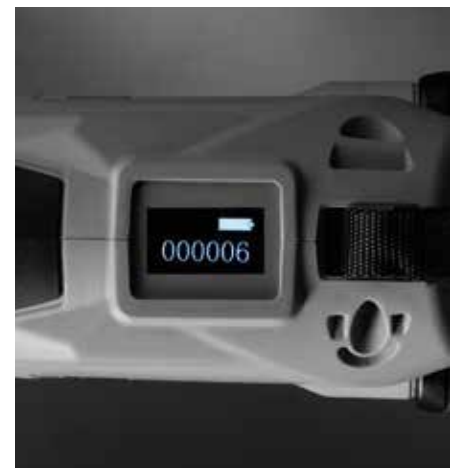
The display provides information about the battery level, service status and number of pressings.
