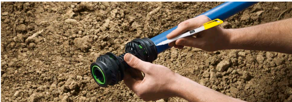
2. Place connector onto pipe. Check the insertion depth in the window and draw a safety mark on the pipe.
