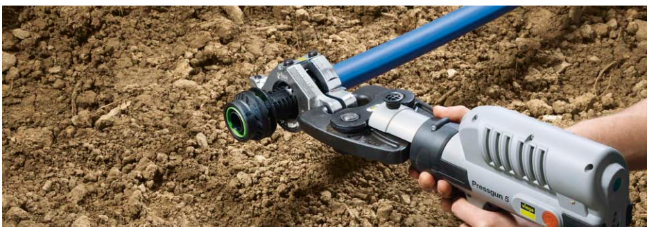
3. Press the connector and check the green pressing marker.
