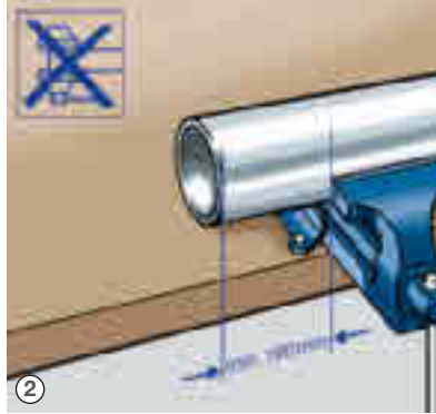
2 Use the vice with caution! The end of the pipe must be perfectly round.
