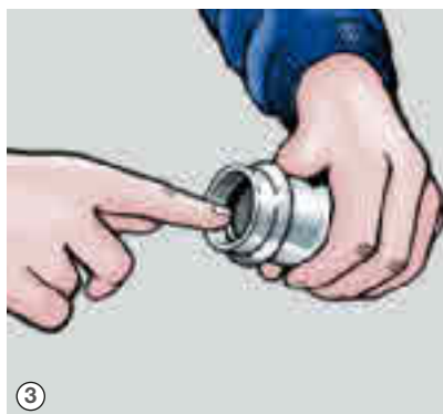
③ Check that the sealing element is seated correctly.
