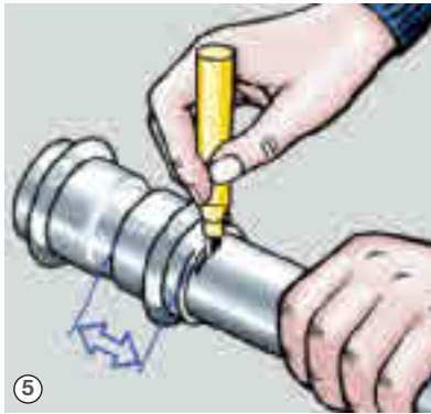
⑤ Mark the insertion depth.
