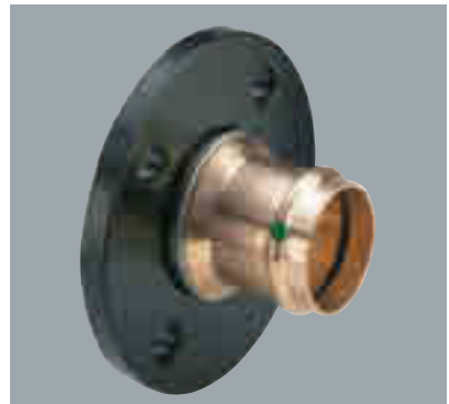
Sanpress Flexible Flange adapter steel, black powder-coated, with gunmetal press connector 28 – 54 mm Model 2259.5 64 mm (copper) Model 2459.5XL 76.1 – 108.0mm Model 2259.5XL
