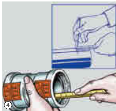
4 Mark the insertion depth. \varnothing 64.0 mm = 43 mm \varnothing 76.1 mm = 50 mm \varnothing 88.9 mm = 50 mm \varnothing 108.0 mm = 60 mm
