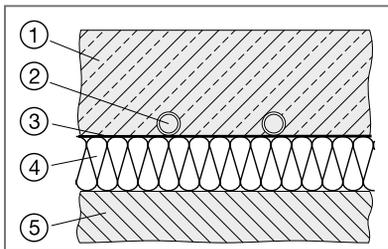
Fig. 100: Systems with pipes within the screed
