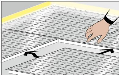
Fig. 103: Join the insulation panels, press the overlapping marking area in. Avoid cross joints.
