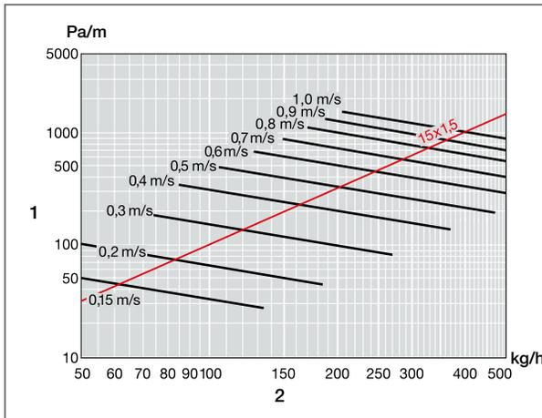
Fig. 85: Pressure loss diagram PB pipe 15 x 1.5 mm
