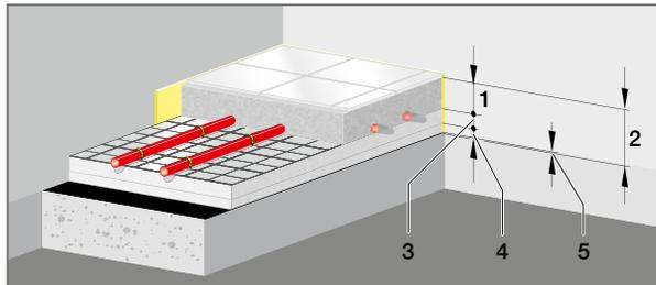
Fig. 83: Installation situation II + III + V according to DIN EN 1264-4
