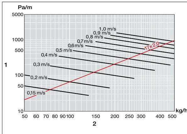
Fig. 90: Pressure loss diagram PB/PE-Xc/PE-RT 17x2.0mm
