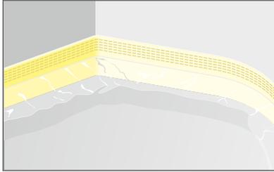
Fig. 101: Lay and fasten the edge insulation strips.
