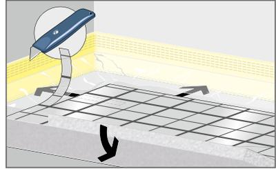
Fig. 102: Trim off any protruding marking foil, unfold and lay the heat/footfall sound insulation.
