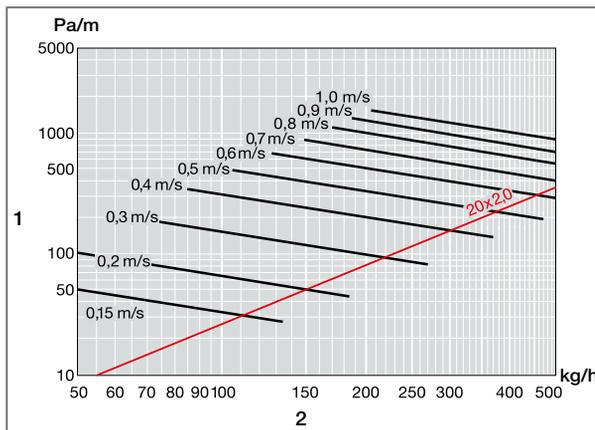
Fig. 95: Pressure loss diagram PB/PE-Xc/PE-RT 20x2.0mm
