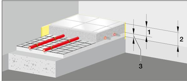
Fig. 82: Installation situation I according to DIN EN 1264-4
