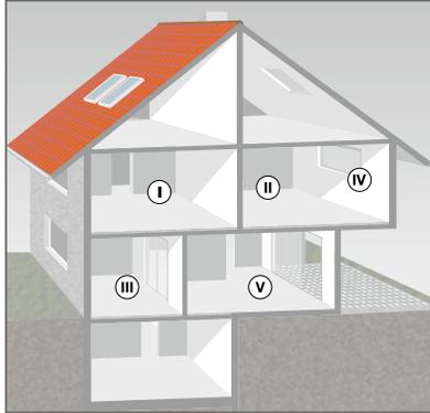
Fig. 81: Installation situations according to DIN EN 1264-4
