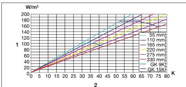
$R_{\lambda,B} = 0.15 \text{ m}^2 \text{ K/W}$
