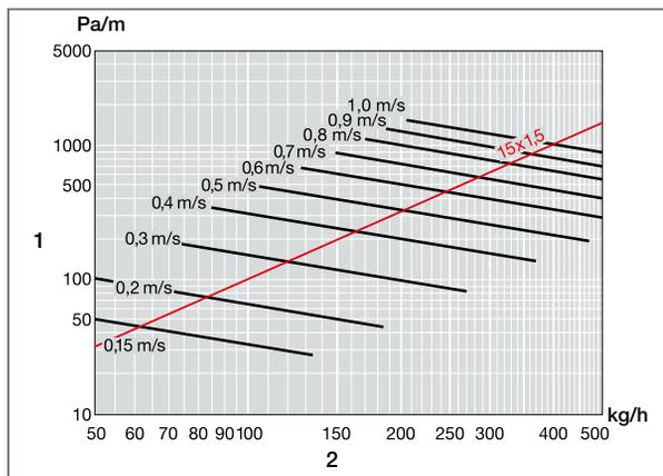
Fig. 59: Pressure loss diagram PB pipe 15 x 1.5 mm
