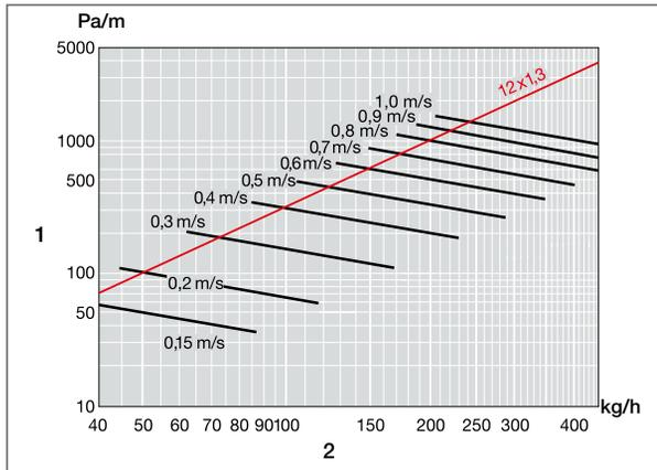
Fig. 54: Pressure loss diagram PB pipe 12x 1.3 mm
