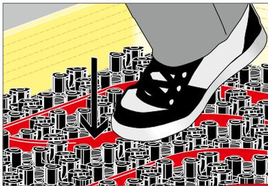
Fig. 75: Lay the heating pipes.
