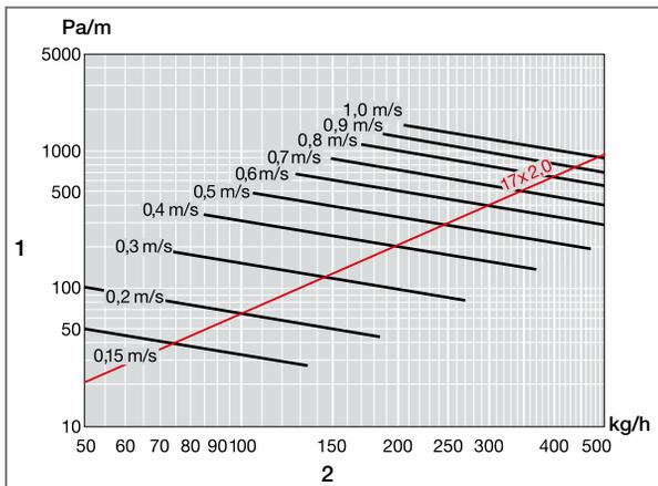
Fig. 64: Pressure loss diagram PB-PB pipe, PE-Xc and PE-RT 17 x 2.0 mm
