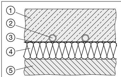
Fig. 69: Systems with pipes within the screed
