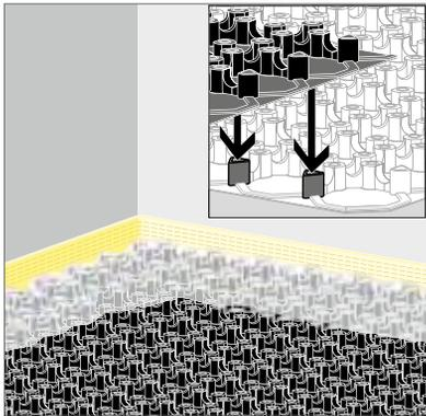
Fig. 73: Lay the snap plate.
