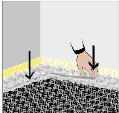
Fig. 74: By means of an edge profile, fix the foil of the edge insulation strip free of tension on the snap plate.
