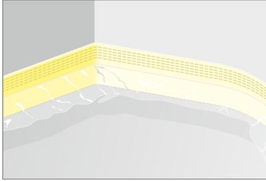
Fig. 71: Lay and fasten the edge insulation strips.
