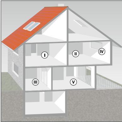
Fig. 50: Installation situations according to DIN EN 1264-4
