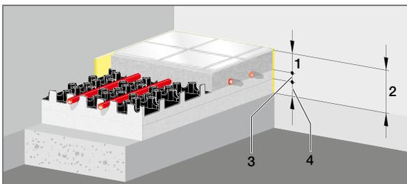
Fig. 53: Installation situation IV according to DIN EN 1264-4
