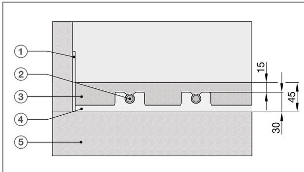
Fig. 29: Total height 45 mm
