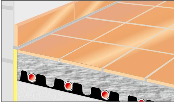
Fig. 46: Natural or artificial stone coverings as floor covering
