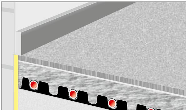
Fig. 47: Textile/elastic floor coverings
