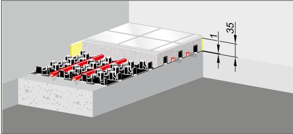
Fig. 30: Floor structure Base Flat 12 with Fonterra Base snap plate, smart
