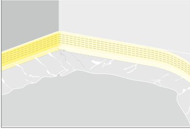
Fig. 40: Lay and fasten the edge insulation strips.
