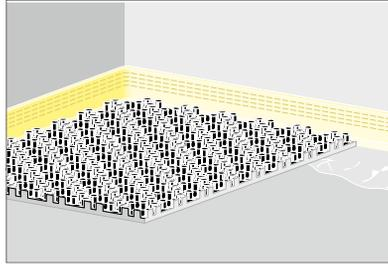
Fig. 41: Lay the Fonterra Base snap plates from left to right. Arrange the film flaps under the snap plate.
