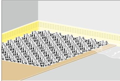
Fig. 43: Laying the Fonterra Base snap plates free of hollow spaces over the entire surface. Arrange the film flaps under the snap plate.
