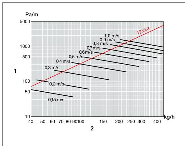
Fig. 32: Pressure loss diagram PB pipe 12 x 1.3 mm
