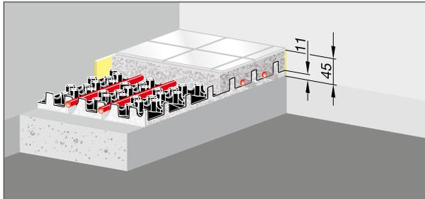
Fig. 28: Floor structure Base Flat 12 with Fonterra Base snap plate, ND 11
